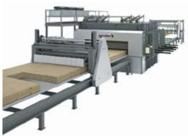
Figure B2.4 Kallasøe timber press
