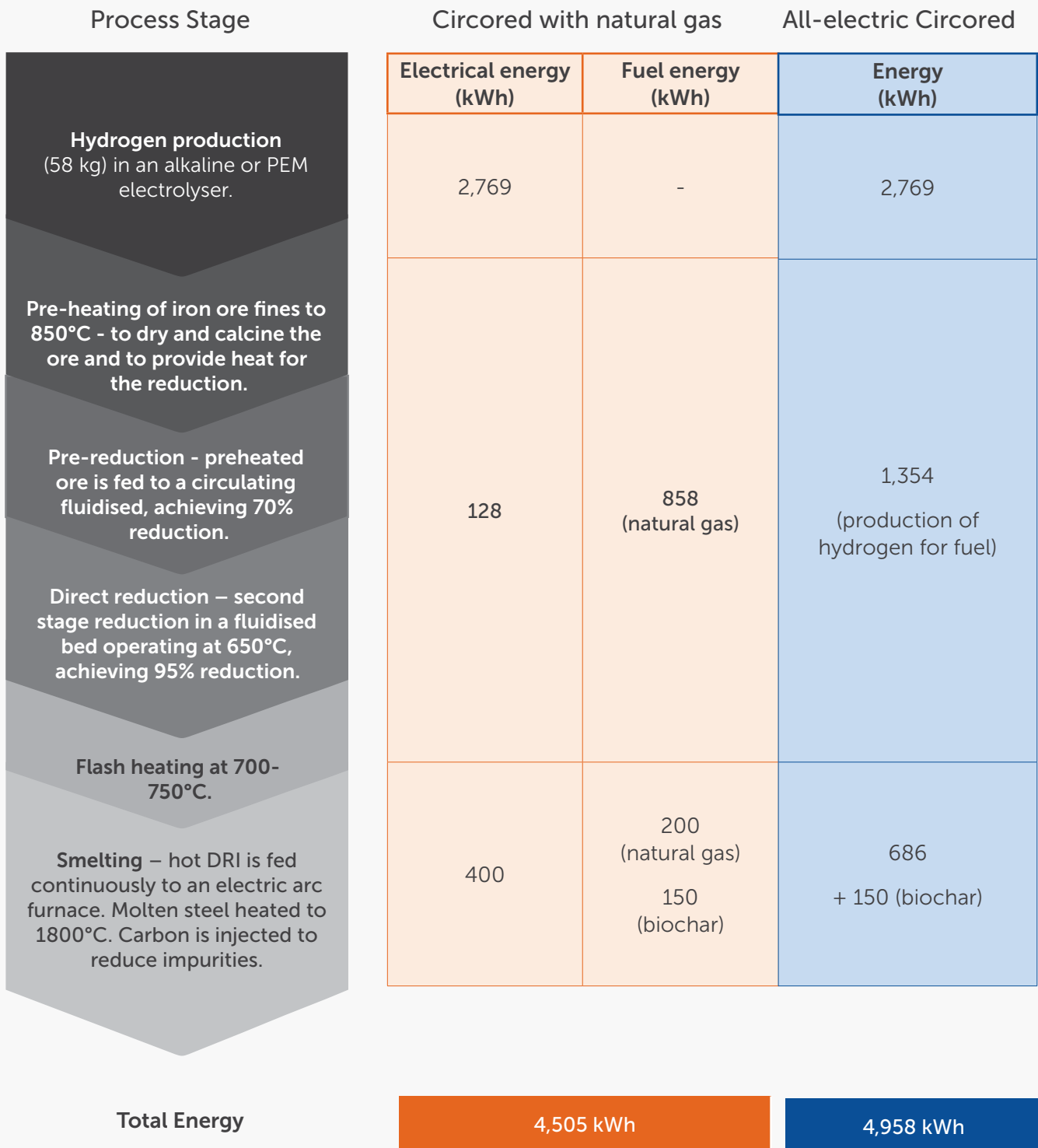
Figure C9.3 Energy requirements to produce 1 tonne of crude steel through direct reduction with hydrogen 273
